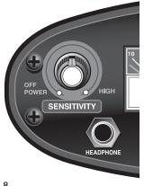
Sensitivity will be reduced slightly when using the Tracker IV in the Discrimination mode. If you want optimal depth capability, operate in the All Metal mode by turning the Discriminate control completely counterclockwise; then turn the Sensitivity control clockwise to its highest clockwise position without chatter. If your Tracker IV chatters or beeps erratically, reduce the Sensitivity by turning the left knob counterclockwise.
